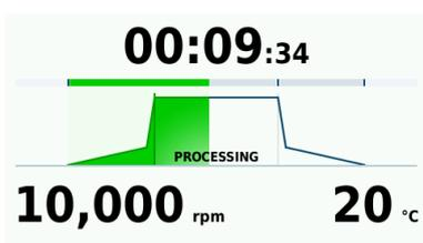
Centrifugation is taking place at the set speed. The time remaining for centrifugation is displayed.
