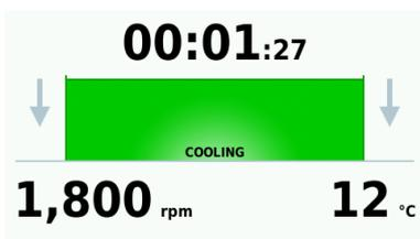
The rotor has been installed and the centrifuge door is closed; precooling in progress. The remaining time for cooling is displayed (see “Precooling” on page 16).
