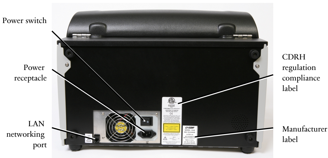
Figure 4-3. Closeup of the Odyssey® DLx Imager rear panel showing the power receptacle and LAN port (use only the supplied networking cable). Also shown are the CDRH regulation compliance label, the manufacturer label and the power switch. The power switch should be left in the 'on' position. Note: The appearance of your instrument's back panel may vary slightly from the one shown.
