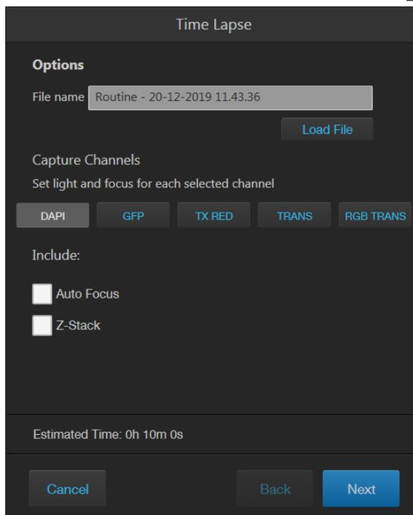
2. Select the **Capture Channels**. You can select multiple channels in which to capture time lapse images. In the following example, **DAPI** and **TX Red** channels have been selected.
