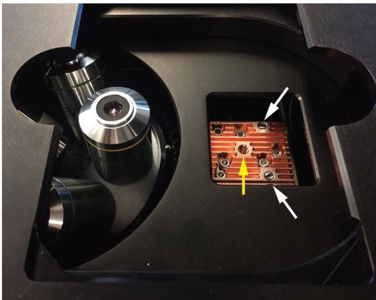
3. Use the light cube tool to loosen the two slotted screws (white arrows) that are flush with the ridges on the light cube.
