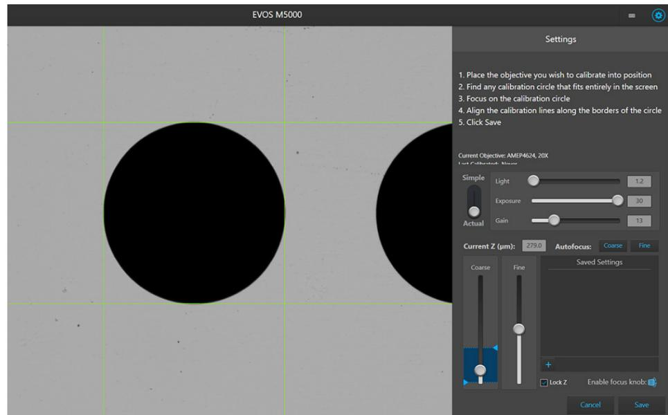
7. When finished, click **Save** to complete the calibration. Repeat the calibration process for each additional objective to be calibrated.
