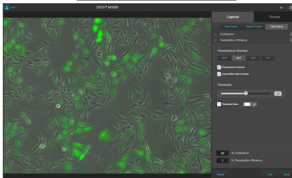
The software automatically calculates the Transfection Efficiency and displays the results as % Confluence and % Transfection Efficiency.
