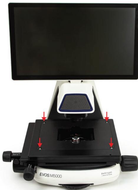
2. Secure the onstage incubator master plate to the X-Y stage using the four thumb screws.
