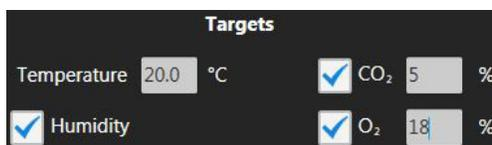
Incubator status will change to “Running” and the control panel will display the Target and Actual values for Temperature, Humidity, CO<sub>2</sub>, and Oxygen.
