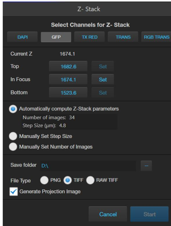
2. Select the **Channels for Z Stack** that you want to capture. You can select multiple channels. In this example, **GFP** channels is selected.
