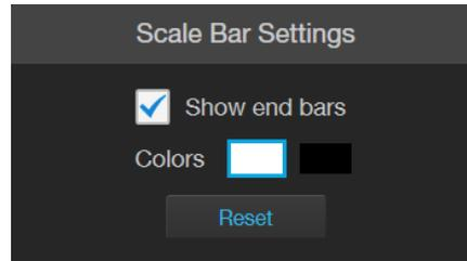
3. Select **Show End Bars** to display the scale bar with the end bars.
