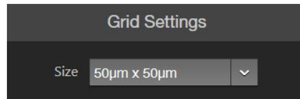
3. Select the **Size** for the grid. Available grid sizes depend on the magnification of the selected objective.
