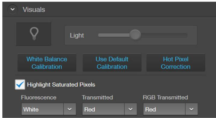
2. To assign a specific color to the saturated pixels in a channel, select the desired color from the corresponding channel dropdown (**Fluorescence**, **Transmitted**, or **RGB Transmitted**).
