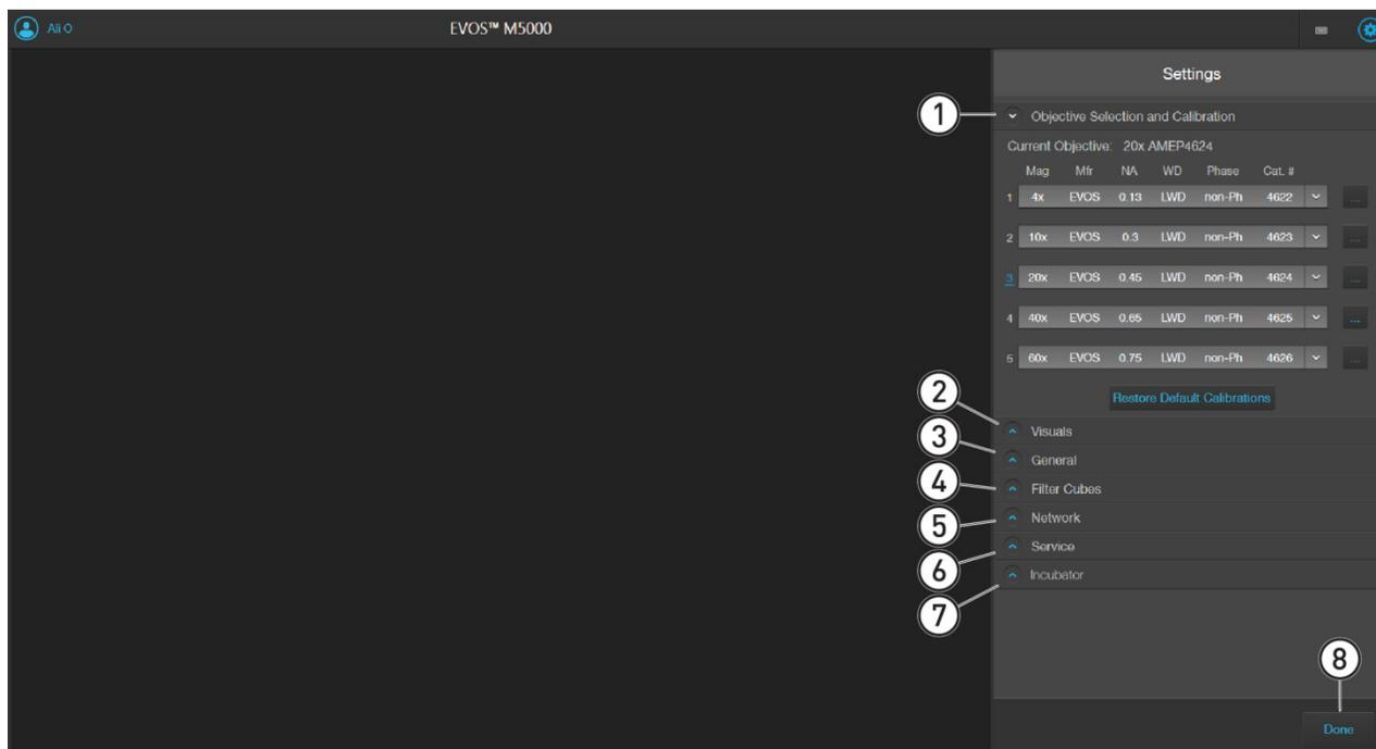
① **Objective Selection and Calibration:** Allows you to assign and unassign objectives on the objective turret, and to calibrate objective magnification.
