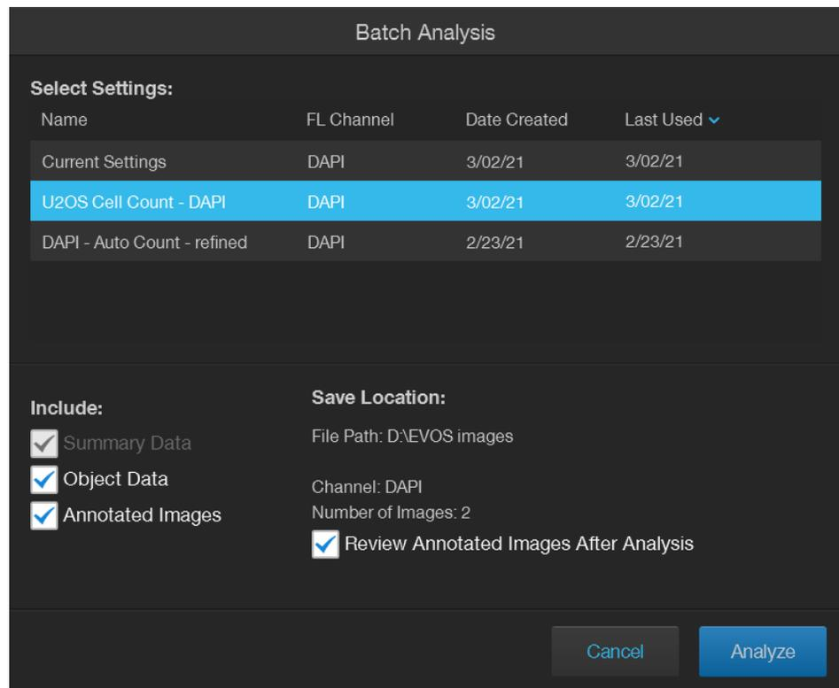
5. To save the **Intensity, Area, and Circularity** data of objects counted in Auto Count, select **Object Data**. When Object Data is selected, the data is saved as separate CSV files for each analyzed image in the analysis folder. The option to save Object Data is available only for Auto Count.
