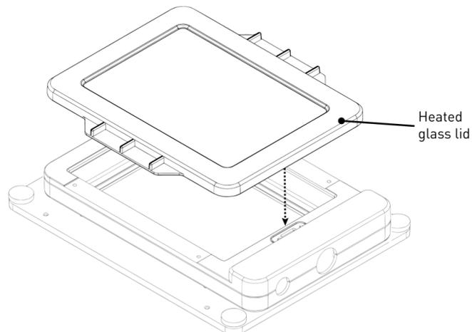
4. Place the light shield with tinted plastic window on top of the heated glass lid. **Use of the light shield is required for fluorescence imaging applications.**
