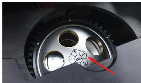
2. Screw the new objective into the open position in the objective turret. Note the part number of the objective and the turret position. In this example, the new objective is installed into the turret position 5.
