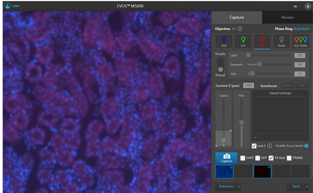
A thumbnail of the image captured in the new channel is displayed along with the thumbnail of the image from the previously captured channel.
