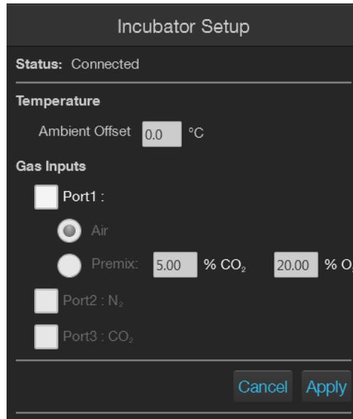
3. Select the appropriate options for the **Gas Inputs** that reflects your set-up for the EVOS™ Onstage Incubator.
