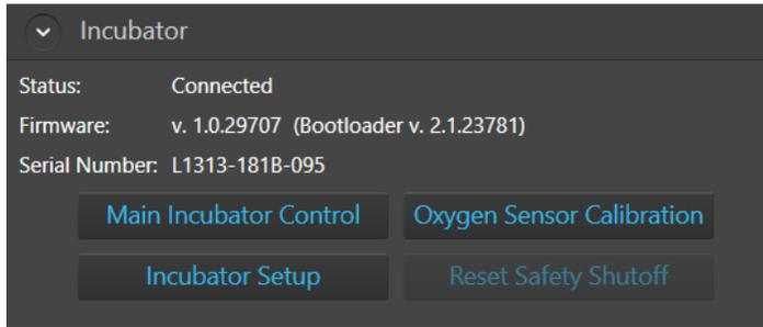
2. Click **Oxygen Sensor Calibration** to open the Incubator Setup window.
