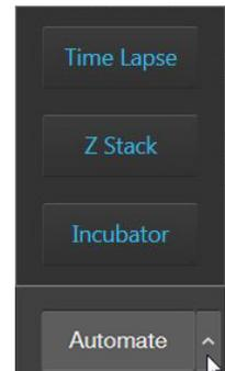
**Time Lapse:** Opens the Time Lapse tool, which allows you to create and run time lapse routines to capture images at given intervals over a time period based on your specifications.
