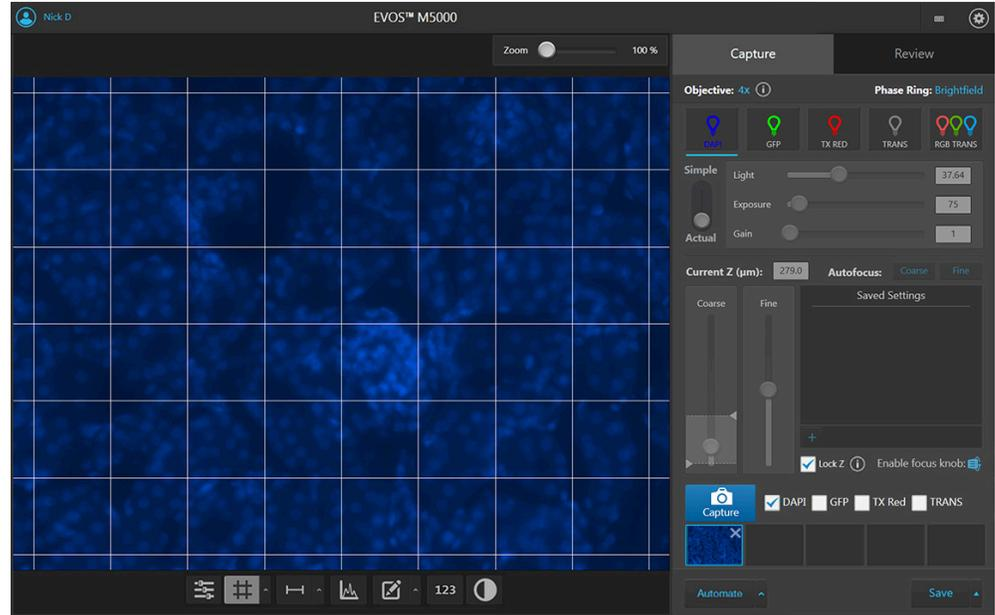
2. To change the grid size, click the **Grid Settings** button (arrow on the Grid split button) to open the Grid Settings tool.
