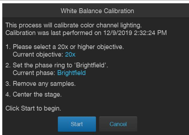
2. Select a 20X or higher objective, then set the phase ring to **Brightfield** using the Phase annuli selector (page 8).
