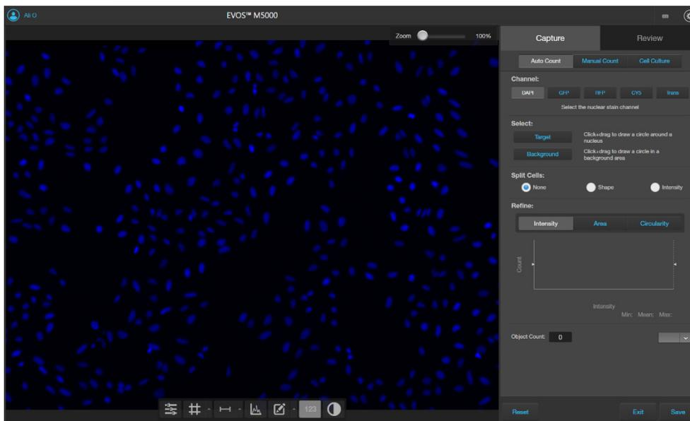
2. If counting from the Capture tab, select the **Channel** in which to count objects. Available options depend on the channels used when the image was captured. In this example, all channels contain captured images, and DAPI is selected for auto count.
