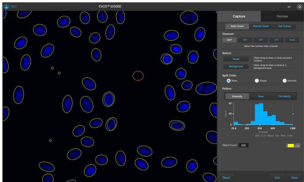
The target objects that were counted are identified with colored circles (in this example, yellow) and the Object Count field displays the number of objects included in the count.
