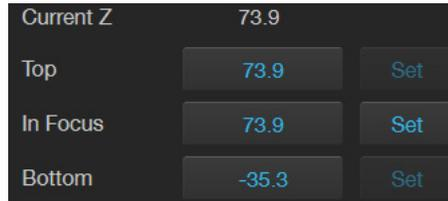
To change the **In Focus** position, move the **Coarse** and **Fine focus** sliders on the Capture tab to focus on the sample, then click **Set**.
