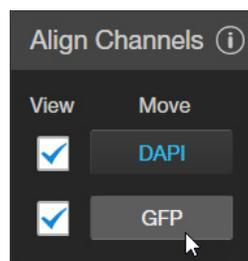
3. *Optional:* To remove a channel from displaying in the Viewing Area, unselect the corresponding **View checkbox**.
