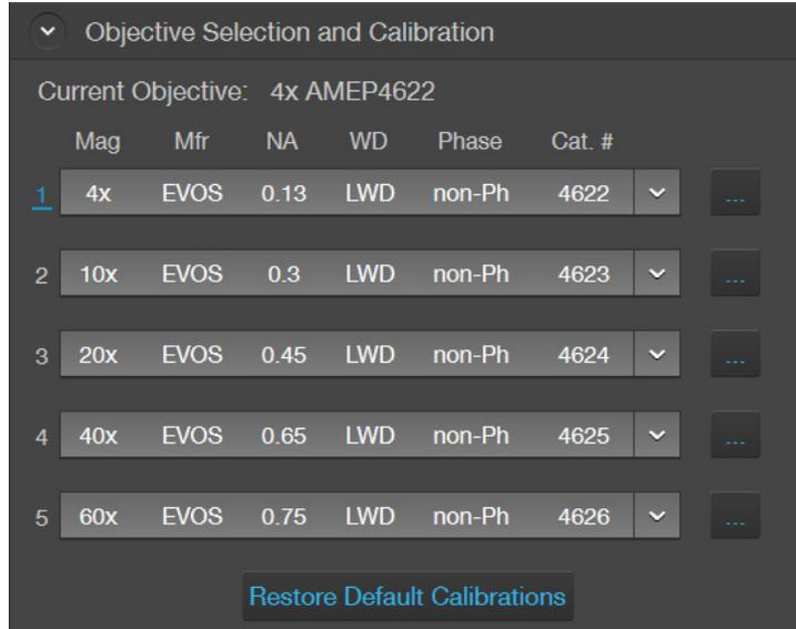
2. Find the newly installed objective in the **Objectives** list for the corresponding turret position.
