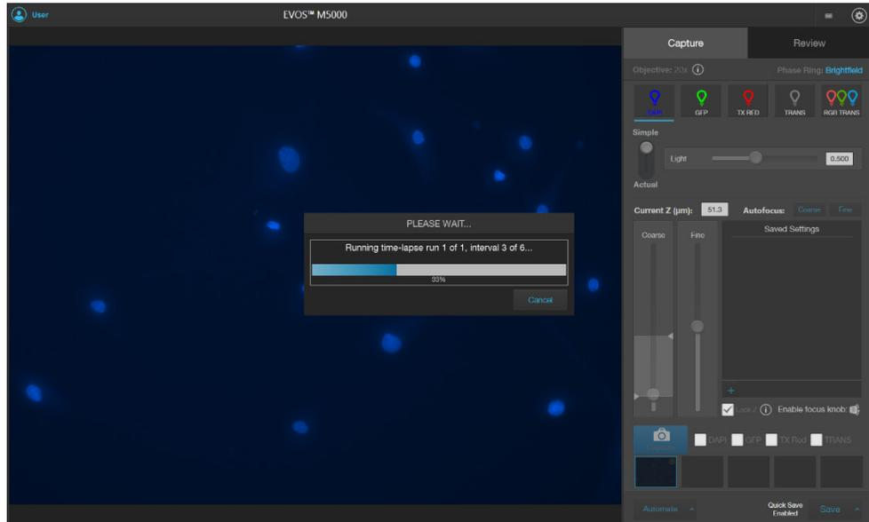
24. When the Time Lapse routine is completed, the Review tab opens to the files captured in the routine.
