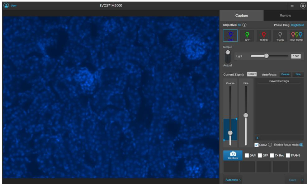
**Note:** You can only select a single light source for Live mode when adjusting brightness and focus. However, you can display and capture multiple channels simultaneously.
