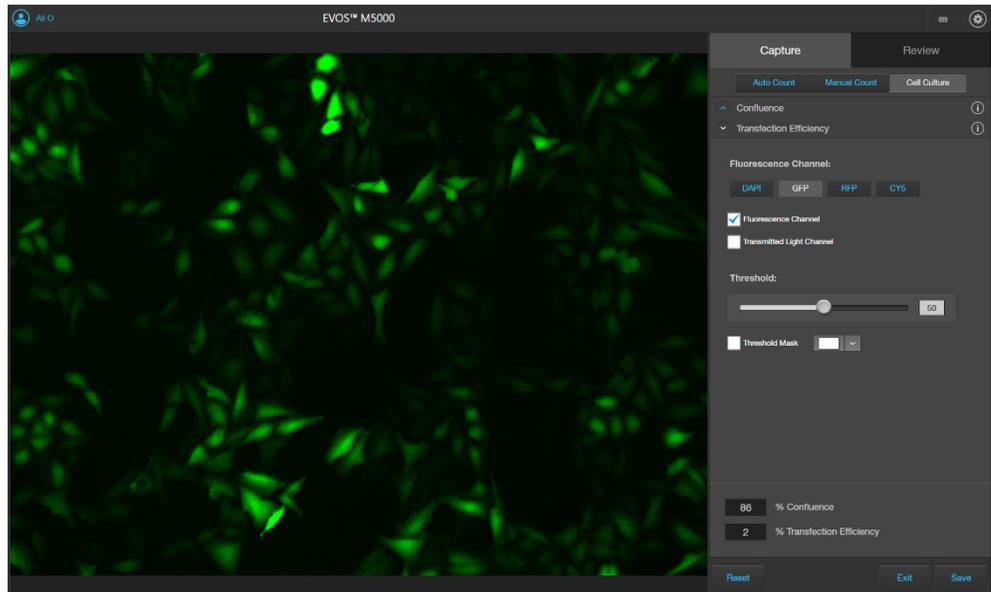
4. Select **Threshold Mask** to highlight the fluorescence areas included in the Transfection Efficiency calculation.
