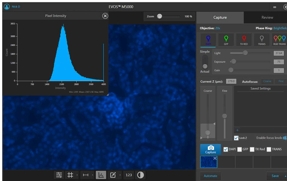
2. The Pixel Intensity histogram shows the Pixel count vs. Intensity data of the image displayed in the Viewing area as well as the minimum, mean, and maximum pixel intensities.
