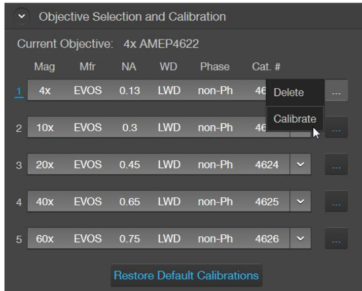
2. Mount the EVOS™ Calibration Slide in the vessel holder, select the objective you want to calibrate, then click **Calibrate Objective**.
