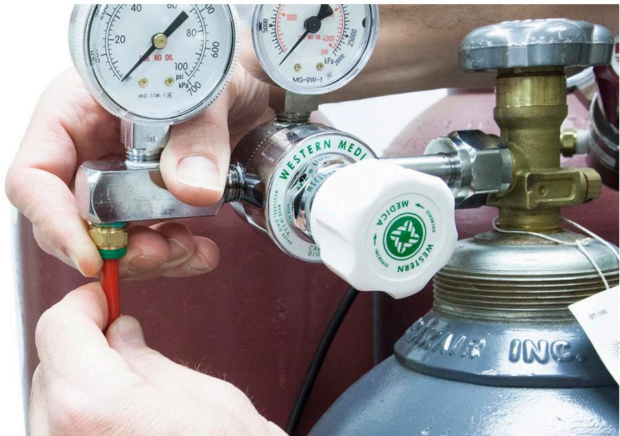
4. Attach the gas lines to the control unit via the PTC connectors for the appropriate gas intake port.
