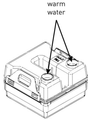
7. Place the water reservoir into the control unit **with the fill holes to the front** and close the lid.
