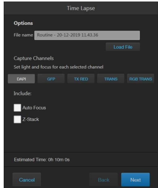
**Z-Stack:** Opens the Z-Stack tool, which allows you to capture multiple images along the Z-axis based on your specifications. You can use the images captured with the Z-Stack tool to generate a Z-Stack Projection.
