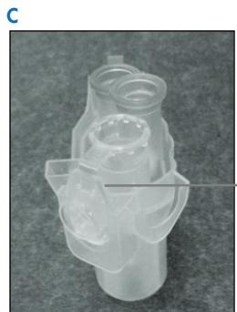
1.5 mL microcentrifuge tube lid not pushed down into slot
