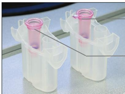
Column lid removed incorrectly; part of the lid is still remaining
