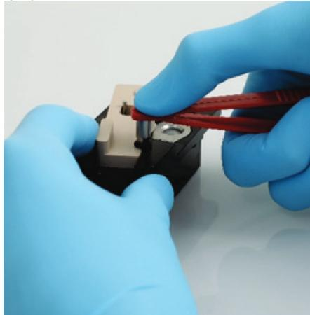
3d. Open the grey lever and insert the peg with small end first into hole as shown.
