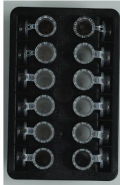
Loading the shaker rack with sample tubes that have attached lids
