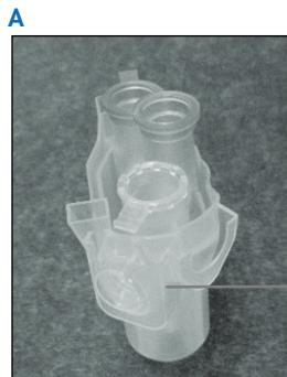
1.5 mL microcentrifuge tube lid is in correct position
