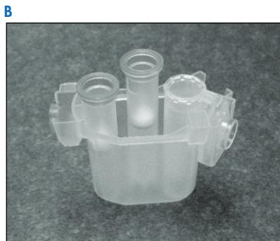
**Correctly loaded rotor adapter.** **A** Rotor adapter is correctly loaded, and the 1.5 mL microcentrifuge tube lid is in the correct position; **B** Correctly loaded rotor adapter seen from the side.
