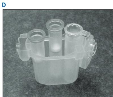
**Incorrectly loaded rotor adapter.** **C** Rotor adapter is incorrectly loaded with a 1.5 mL microcentrifuge tube. The lid of the tube is not pushed all the way down to the bottom of the slot of the rotor adapter and could break off during centrifugation (compare with part A of the above figure); **D** Incorrectly loaded rotor adapter seen from the side (compare with part B of the above figure).
