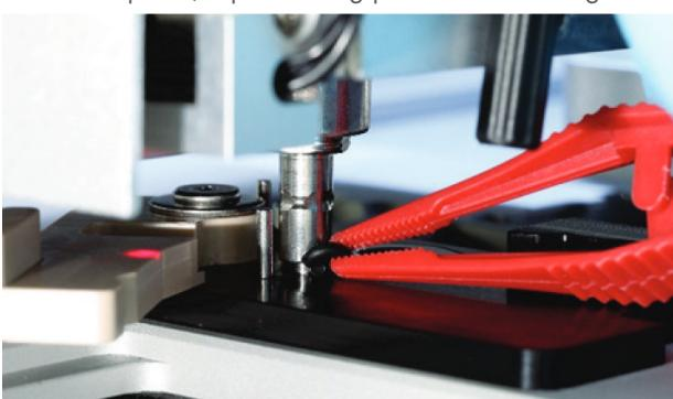
8. Close the hood and press **Next** to pick up the prepared new O-Ring.
