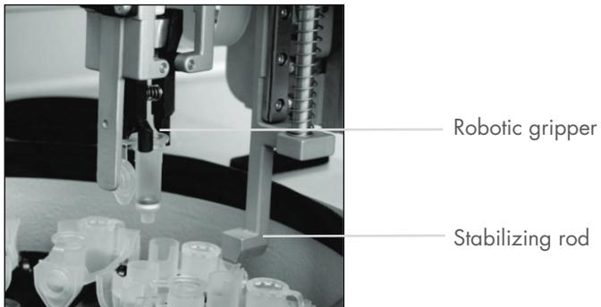
**Robotic gripper automates spin-column processing**
