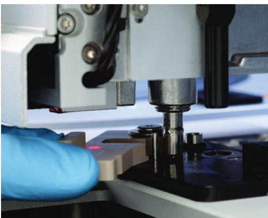
7b. Open the grey lever and remove the O-Ring (by using the tweezers) from pipetting channel.
