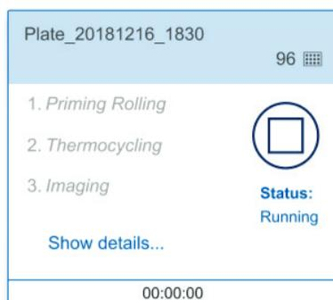
Aborting a plate during the priming/rolling step renders it unusable and the plate cannot be used and run again. A plate that has been aborted during the Thermocycling or Imaging step can be used again. To rerun the plate, configure a run with only the remaining steps. See section Rerunning a plate for more information.
