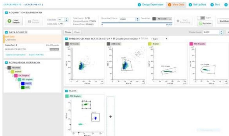
2. Use the **Acquisition Dashboard** panel to load and unload samples, adjust flow rate, agitate samples, run a sample line backflush, control the sample injection chamber light, and record data.
