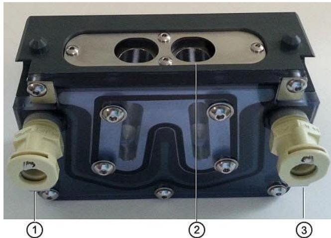
Attach the input tubing to the one port (1 or 3) and the output tubing to the other port (3 or 1).
