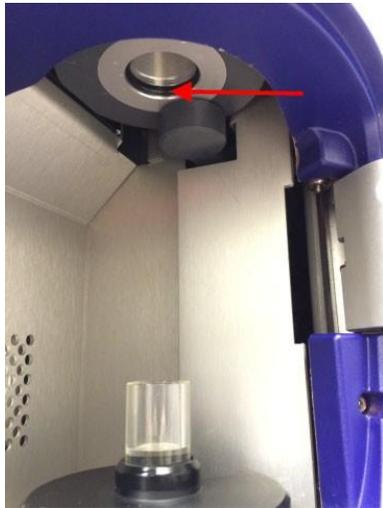
4. If the O-ring is dry, apply a small amount of O-ring lubricant to the O-ring.
