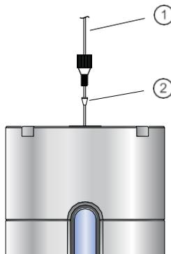
**Note:** If the ferrule is left behind in the injection chamber fitting, gently push the tip of the ferrule-removal tool into the top of the ferrule and pull the ferrule straight out.
