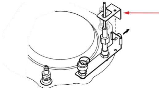
7. Finish loosening the 11/16-inch nut at the top of the probe and pull the probe straight up and out of the sheath tank.
