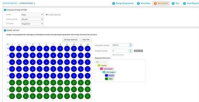
5. Select the initial buffer volume that will be added to each tube or well before sorting.
