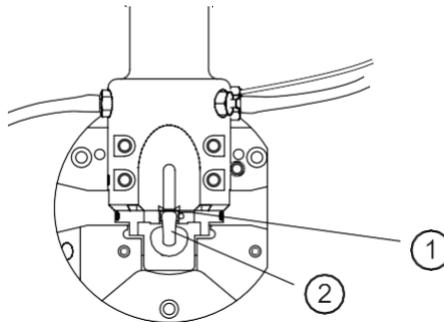
3. Insert the new closed-loop or sort nozzle into the flow cell (with the top side facing up) and push it gently all the way forward until it stops.
