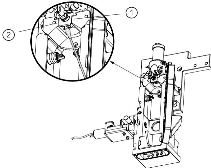
6. Gently wipe the upper camera window and the strobe lens (opposite the window) to remove any saline.
